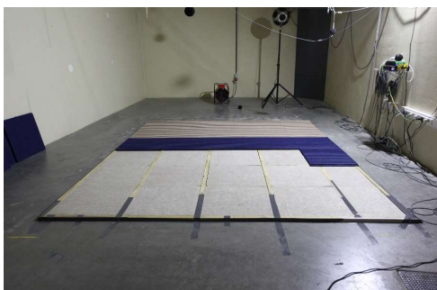
photo : Test n° 22 : during placement of the panels on the frame filled with rockwool
