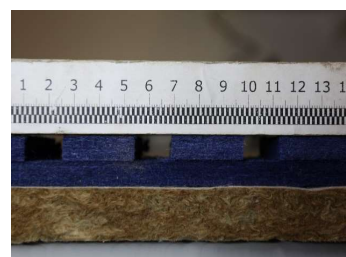
photo: Test n°21: detail of the cross section of the SlimWall panels of 18 mm on the rockwool panels of 20 mm
