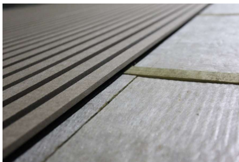
photo : Test n° 22 : details during placement of the SlimWall Lines panels on the wooden frame with a height of 22mm and filled with 20 mm rockwool.
