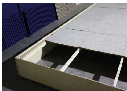
photo: Test n° 21 : during placement of the rockwool panels on the empty frame of 270 mm
