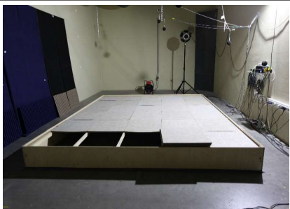
photo: Test n° 21 : during placement of the rockwool panels on the empty frame of 270 mm
