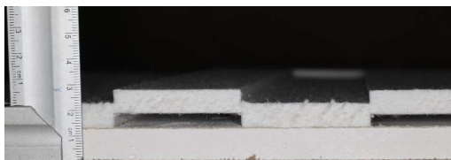
photo: Section view of the felt wallcovering glued to a gypsum board
