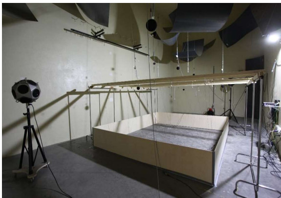
photo : Empty reverberation room with non-absorbent frame for measurement setup
