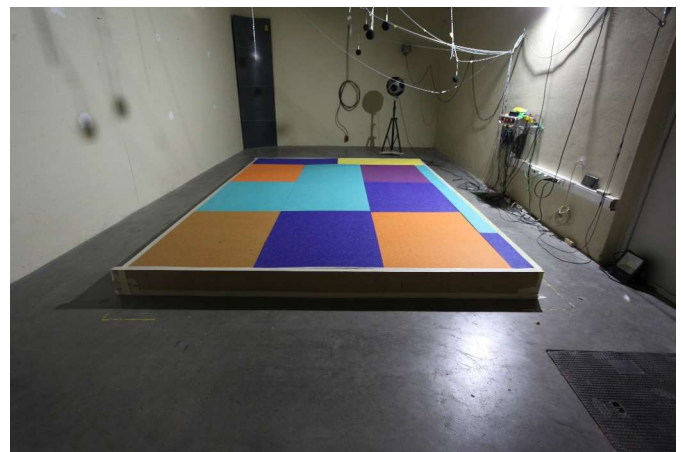
photo : test arrangement SlimPanel 9mm with air gap of 191mm Type E-200 mounting
