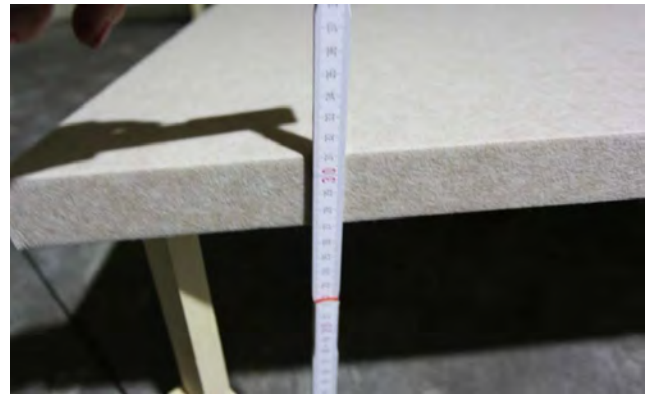
photo : side view of the test object: ceiling island on wooden supports, with a height of 270mm
